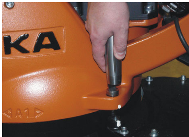
Fig. 5-7: Removing protective cap from gauge cartridge
